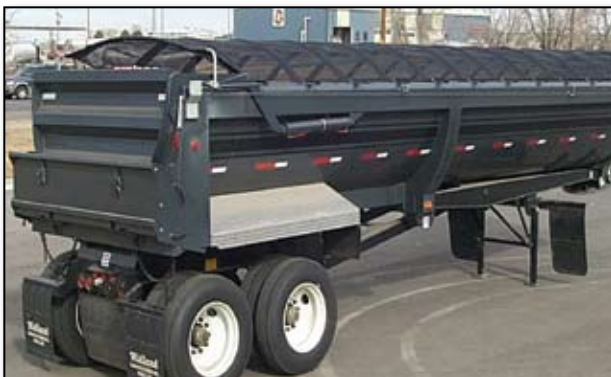
Front to Back Cable System with Heavy Duty Mesh
