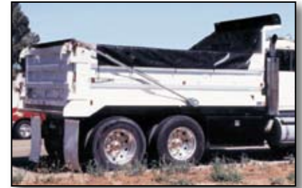
Automatic Arm System with Asphalt Material and patented ground operated Flap System.
