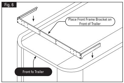
**Step 6**: Place the front frame bracket assembly on the front of the trailer. Align the assembly making sure that the brackets are parallel to the trailer and each other. The entire assembly must be square to the trailer and level. Clamp in place (Fig. 6).
