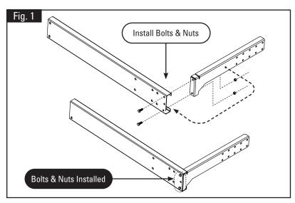
**Step 1:** Bolt 24" Left Mount Bracket (502-0714) to the Outer Channel Mount (502-0170, driver's side) using two 3/8" bolts (503-3704) and nuts (504-3702) provided (Fig. 1).
