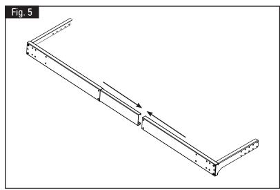
**Step 5**: Slide the Outer Channel Mount (502-0170, driver's side) over the Inner Channel Mount (502-0169). Adjust the assembly so that the 24" Mount Brackets are the same distance apart as the width of the trailer. Clamp the Inner and Outer Channel Mounts together to hold in position (Fig. 5).
