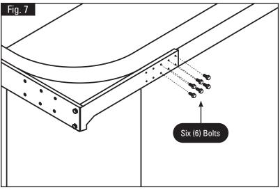
**Step 7**: Weld or bolt the 24" Mount Brackets to the trailer. A 21/64 pilot hole must be drilled first when using the 3/8" - 16 x 1.25", (503-3705) self threading bolts that are provided. Six bolts per side are adequate for most installations (Fig. 7).
