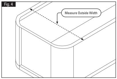
**Step 4:** Measure the outside width of the trailer at the front where the bracket assembly will be mounted (Fig. 4).
