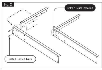
**Step 2**: Bolt 24" Right Mount Bracket (502-0715) to the Outer Channel Mount (502-0171, passenger's side) using two 3/8" bolts (503-3704) and nuts (504-3702) provided (Fig. 2).
