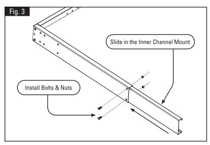
**Step 3:** Slide the Inner Channel Mount (502-0169) into the Outer Channel Mount (502-0171, passenger's side). Line up the holes and bolt in place using two 3/8" bolts (503-3704) and nuts (504-3702) provided (Fig. 3).
