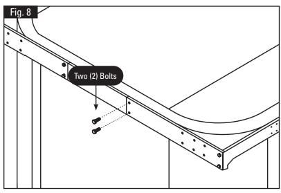
**Step 8:** Remove the clamp from step 5 and drill two 3/8" holes through the Inner Channel Mount on the driver's side using the holes in the Outer Channel mount as a guide. Line up the holes and bolt in place using two 3/8" bolts (503-3704) and nuts (504-3702) provided (Fig. 8).
