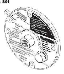
2. Tighten down the ratchet lock bolt firmly.
