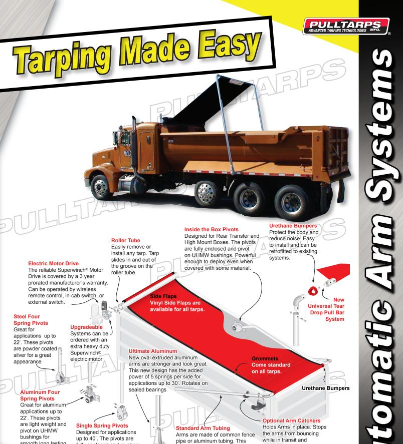
fully enclosed and pivot on UHMW bushings for smooth and long lasting operation
