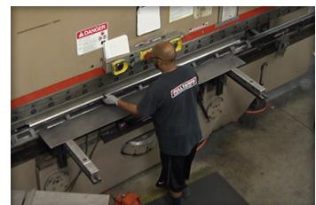
Computer operated brakes form complex shapes perfect for bump rolling our system housings.
