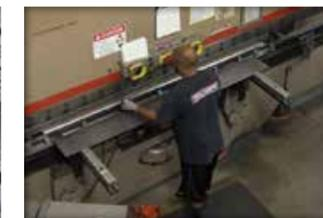
Computer operated brakes form complex shapes perfect for bump rolling our system housings.
