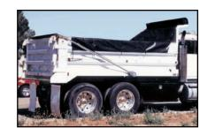
Automatic Arm System with Asphalt Material and patented ground operated Flap System.
