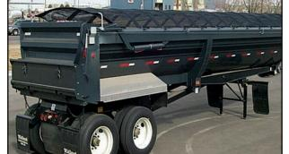
Front to Back Cable System with Heavy Duty Mesh
