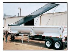
Electric Arm System with Heavy Duty Mesh
