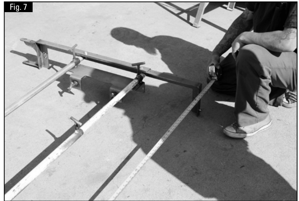
Step 7: Loosen the T bolts and adjust the width (Fig. 7).
