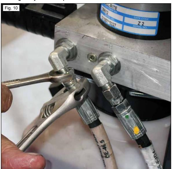
Step 7: Attached the second Hydraulic line (Marked Red) to the second (outer) Hydraulic connector (Fig. 10).
