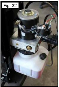
**Step 29:** After filling, reinsert filler cap and secure. Check system for leaks. (Fig. 32).
